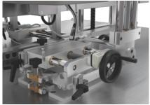
Labelling head support with micrometric adjustment.
